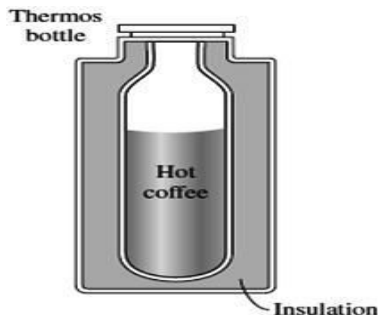
Fig. 1 Heat transfer from the thermos
