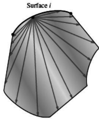
Fig. 20 Radiation leaving the surface i of an enclosure intercepted by completely by the surface of enclosure
