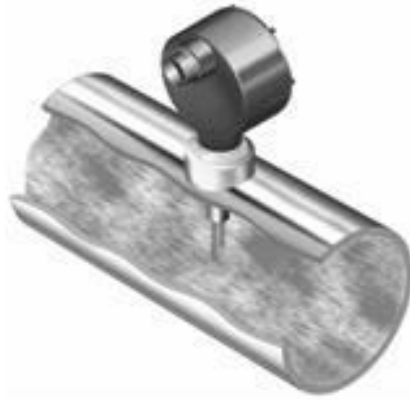
Fig. 8 Use of thermometric well
