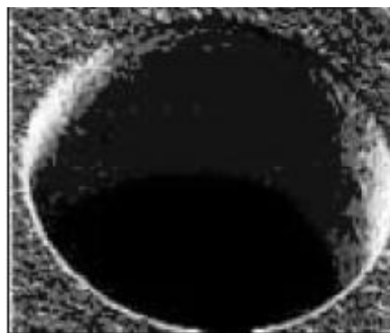
Figure : A non-round hole made by USM
