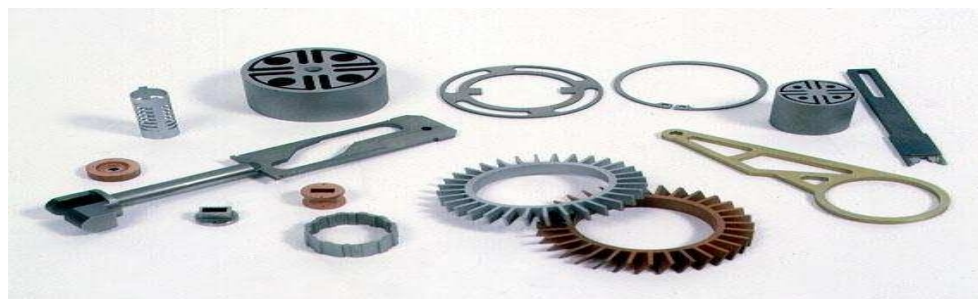
Figure: Difficult internal parts made by EDM process
