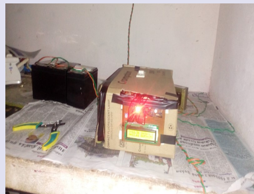
Decentralised PWM based Solar PV lightning System
